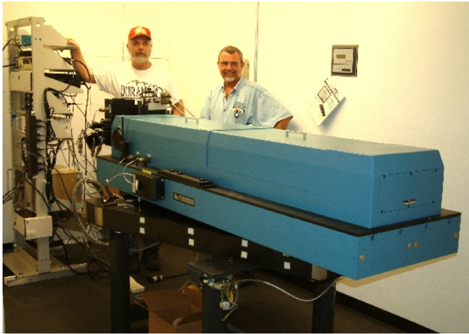
Figure 4.1: The Integrated Sunlight Spectrometer (ISS) installed at the Kitt Peak SOLIS Tower, was relocated after 10 years, in 2014, to the “GONG farm” in Tucson. 4 The light is fed into the instrument via optical fibers (left). 5
